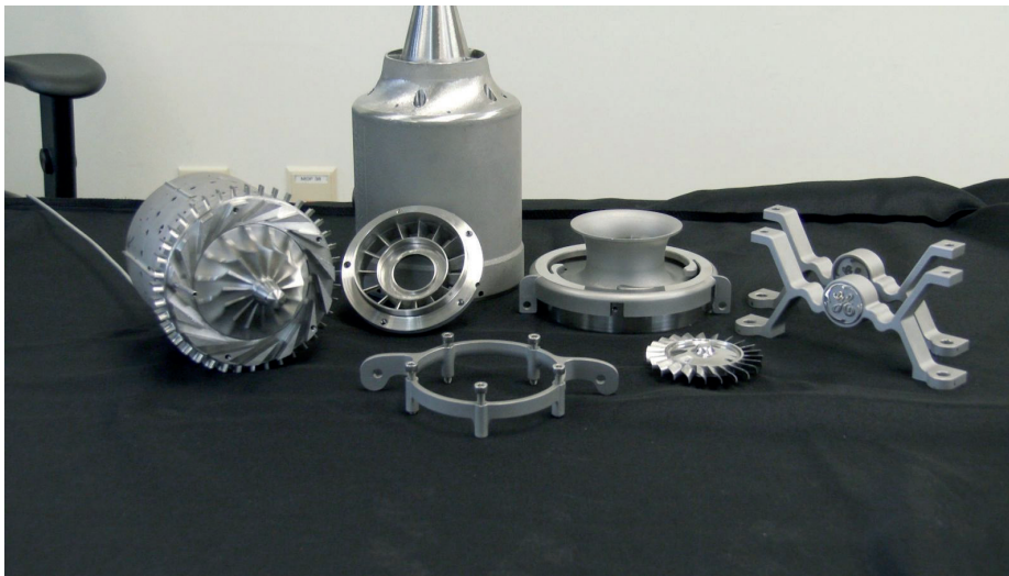
Figure 4: The GE 3D printed working engine prototype.
